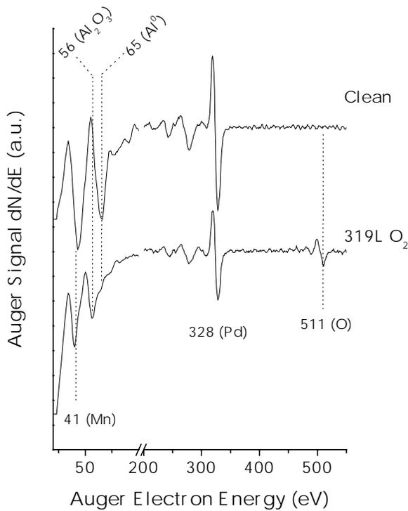
**Figure 1.** Auger electron spectra of the clean  $\text{Al}_{48}\text{Pd}_{42}\text{Mn}_{10}$  surface (upper) and the same surface saturated with oxygen (lower). The clean surface spectrum exhibits peaks from the three components of the alloy: Al at 65 eV, Pd at 328 eV, and Mn at 41 eV. Once oxidized a peak due to O appears at 511 eV. Also note that the Al peak shifts to 56 eV as a result of the formation of a film of aluminum oxide.
