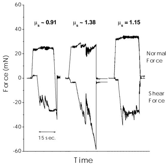
**Figure 3.** Three friction measurements made between clean  $Al_{48}Pd_{42}Mn_{10}$  approximant surfaces. The upper trace is a plot of the normal force, while the lower trace is a plot of the shear force. Friction behavior between the approximants was found to be more erratic than for the quasicrystals. Adhesion can be seen (left trace) as indicated by a negative normal force upon surface separation. Stick-slip friction was also observed for the approximants (middle trace).
