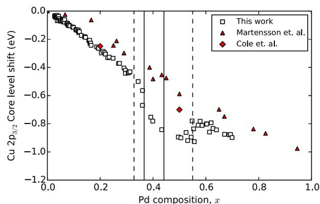
**Fig. 3.** Experimentally measured bulk composition dependent Cu CLS (this work, open squares) compared to previous experimental results (red triangles [12], red diamonds [13]). The solid vertical lines delineate the B2 region, and the dashed lines delineate the mixed region boundaries at 800 K in the experimental phase diagram.
