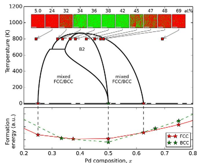
**Fig. 2.** In the top of the figure, electron backscatter phase maps are overlaid on a phase diagram showing the FCC (red) and BCC (green) phase behavior of the CSAF at different compositions [10]. The BCC phases coincide with the known B2 range of the phase diagram at 800 K. In the bottom of the figure are ground state computational structures (stars) compared with their corresponding position on the phase diagram.
