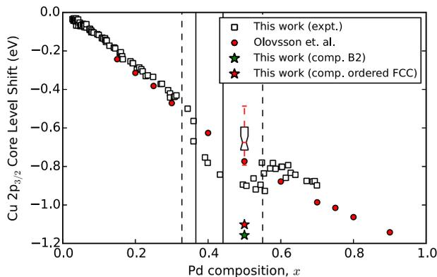
**Fig. 5.** Comparison of peak widening and ground state CLS calculations with the experimental data (open squares) for Cu CLS in  $\text{Cu}_{1-x}\text{Pd}_x$  alloy. Computational work [14] shown in red for randomly configured FCC alloy (circles), for ordered FCC structure (this work, red star) and B2 structure (green star). The bar and whisker plot shows the calculated (this work) distribution of the Cu CLS in a randomly ordered FCC alloy.
