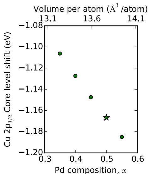
Fig. 7. Effects of lattice constant on the calculated CLS of the ordered B2 phase. The star represents the CLS of the stoichiometric B2 phase at the ground state volume.
