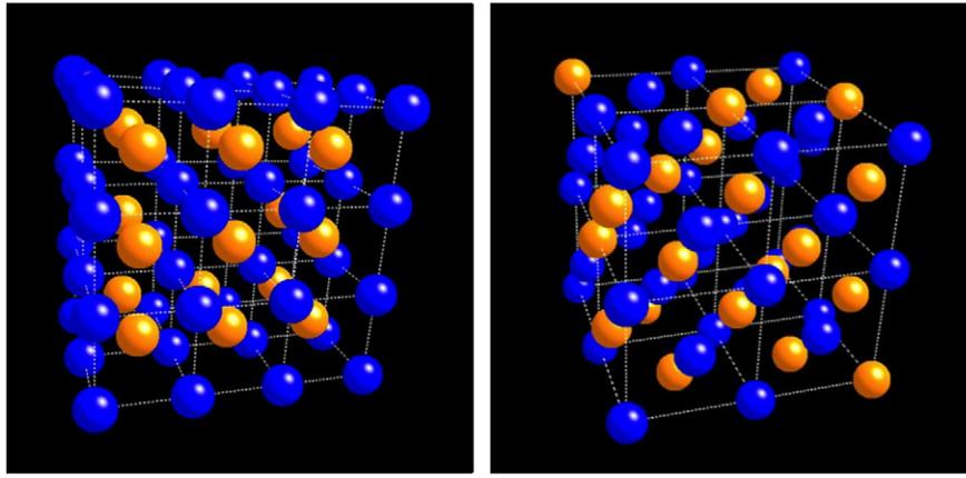
Fig. 1. Left.  $\text{Cu}_{0.5}\text{Pd}_{0.5}$  ordered alloy in the B2 phase at 0 K (Pd – blue, Cu – orange). Right.  $\text{Cu}_{0.3}\text{Pd}_{0.7}$  disordered alloy in the FCC phase.
