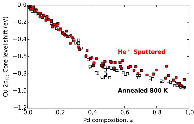
**Fig. 4.** Cu  $2p_{3/2}$  CLS versus  $\text{Cu}_{1-x}\text{Pd}_x$  composition. The Cu  $2p_{3/2}$  CLS measured after  $\text{He}^+$  ion sputtering at 1 keV for 6 min (solid red squares) shows a clear suppression of the CLS associated with the B2 phase. This B2-related CLS reappears after annealing at 800 K for 60 min (open squares).
