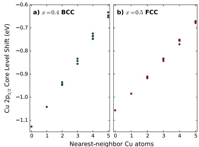
**Fig. 6.** Effect of the number of nearest-neighbor Cu atoms on the calculated CLS of a Cu atom in a) the B2 structure at a lattice constant consistent with 40% Pd and with different numbers of Cu atom nearest neighbors and b) in the ordered FCC structure at  $x = 0.5$  with different numbers of nearest neighbor Cu atoms. There are multiple points for each nearest-neighbor number because there are different local environments.
