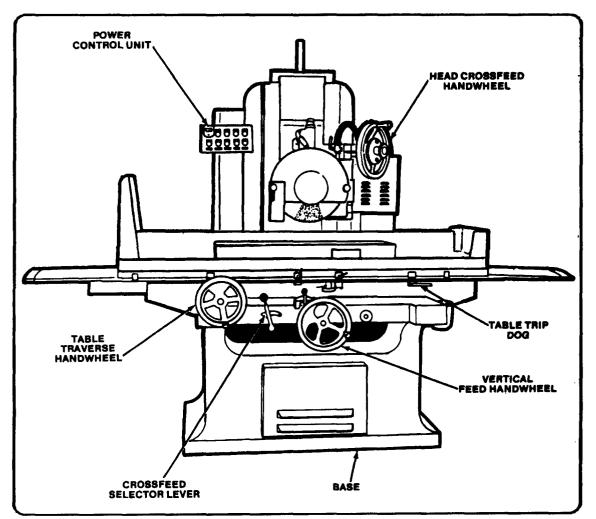
Figure 5-6. Reciprocating surface grinding machine.
