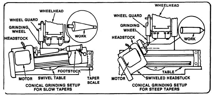
Figure 5-15. Conical grinding setups.
