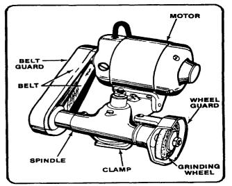
Figure 5-5. Tool post grinding machine.
