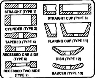
Figure 5-7. Standard types of grinding wheels.
