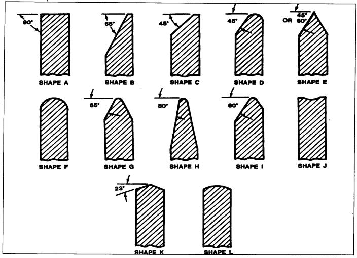
Figure 5-10. Standard shapes of grinding wheel faces.
