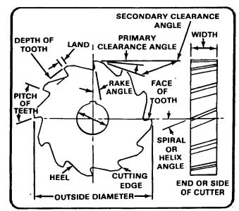
Figure 5-19. Milling, cutter nomenclature.
