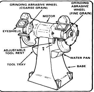
Figure 5-1. Floor-mounted utility grinding machine.
