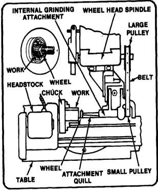
Figure 5-16. Internal grinding setup.
