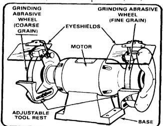
Figure 5-2. Bench-type utility grinding machine.
