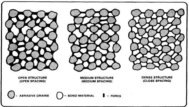
Figure 5-8. Grinding wheel abrasive.
