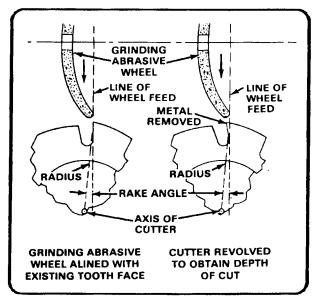
Figure 5-18. Aligning formed milling cutter and grinding wheel.
