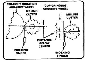
Figure 5-20. Grinding primary clearance angle.
