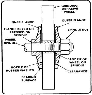
Figure 5-12. Correctly mounted wheel.
