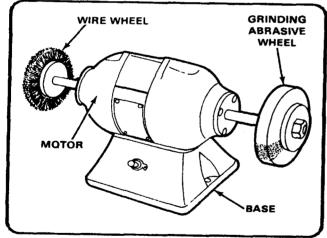
Figure 5-3. Bench type utility grinding and buffing machine
